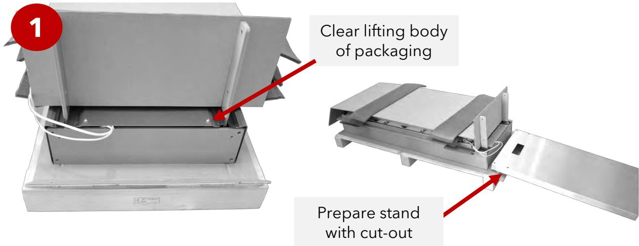
Subsequently, the power cable and the foot switch must be threaded through the cut-out provided in the stand prior to screwing the stand to the lifting body.
