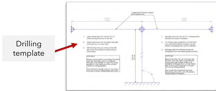
As shown below, the central hole with 145cm (= 57.1 inch) or (if the supplied wall anchors are used for stabilization as recommended - see chapter below) at least 148cm (= 58.3 inch) distance to the floor has to be measured or marked accordingly on the designated wall for mounting the product using the drilling template.
