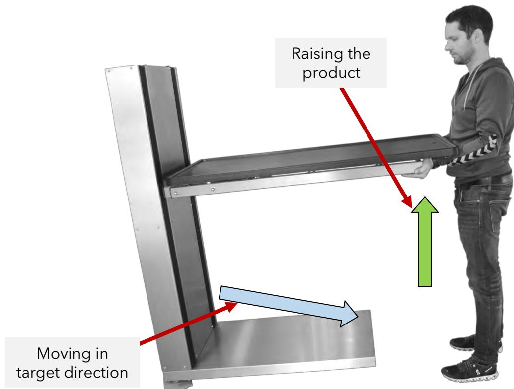
Once the table has reached its target position, lower it again to ensure that the center of gravity is evenly distributed on all four feet.
