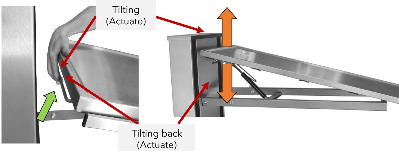
Tilting as well as tilting back (in the opposite direction) is performed by actuating and holding the indicated flap upwards.
