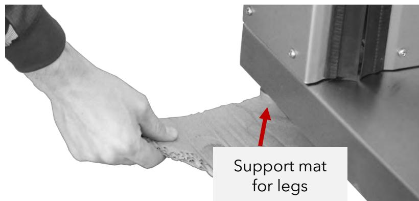
Subsequently, the electrical power cord must be disconnected from the source of electricity. After that, shift the center of gravity of the table by lifting it slightly onto the leveling feet located at the lifting body of the product, such that the product can be maneuvered by applying light force.
