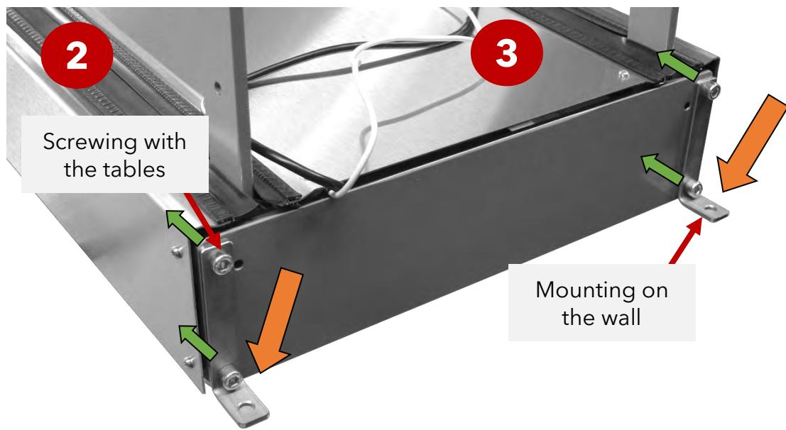
For attaching the anchors to the wall subsequently - as already described above - the local conditions and circumstances must be taken into account accordingly in each case and also the screws and materials required for the wall at hand must be selected accordingly by the customer himself so that stability and load-bearing capacity are ensured.
