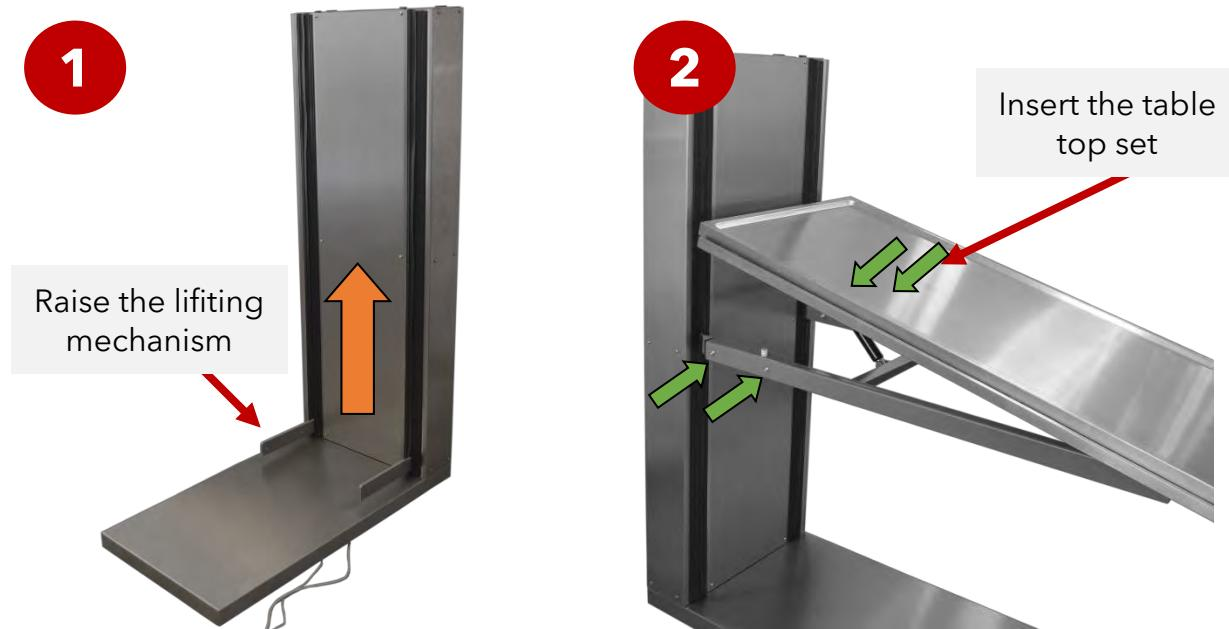
Now, the provided table top set may be positioned on the base frame using the designated 4 screw points. For greater convenience during assembly, the table top set can also be placed on a holder/table in the meantime and the lifting mechanism moved to the appropriate position by actuating the foot switch in order to avoid having to hold the weight of the table top set.
