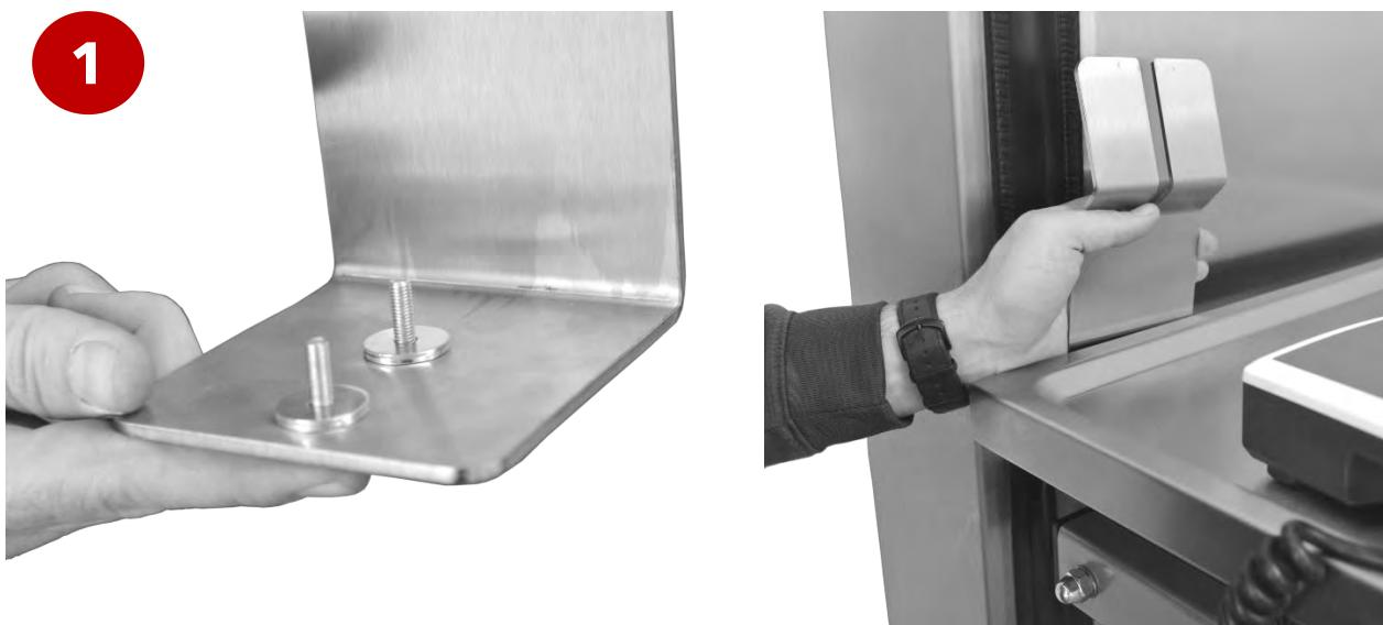
Afterwards, slide the display holder sideways from the left underneath the front side of the table top at the lifting body. Tighten and screw it accordingly from below with the suitable Allen key.
