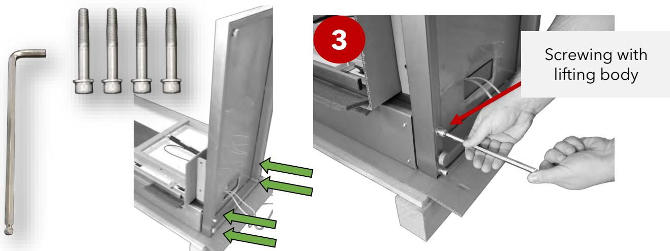
Then take the table off the packaging and transfer the balance weight to the stand before positioning it at the designated place. Be careful not to damage the power cable or the foot switch cable when tilting and transporting the table!
