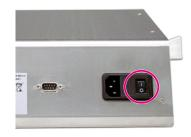
After switching on the sealing device, the display shows the message Heating up. It takes approx. 3-5 min before the pre-set sealing temperature of 180 °C is reached.
