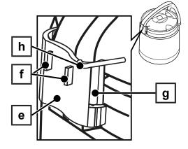
13. Place the holder for spout cover (pos. g) from above onto the holder for the adapter cover. The spout cover can be hooked onto the rear end (pos. h) for safe storage during operation. In addition, the holder fixes the cover of the glass flask to prevent it from falling down.
