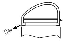
Align the metal collar in such a way that the other screw on the collar lie exactly opposite the spout (pos. a).
