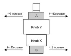
The torque of the y-axis and x-axis travel knobs can be adjusted by torque adjusting knobs.
